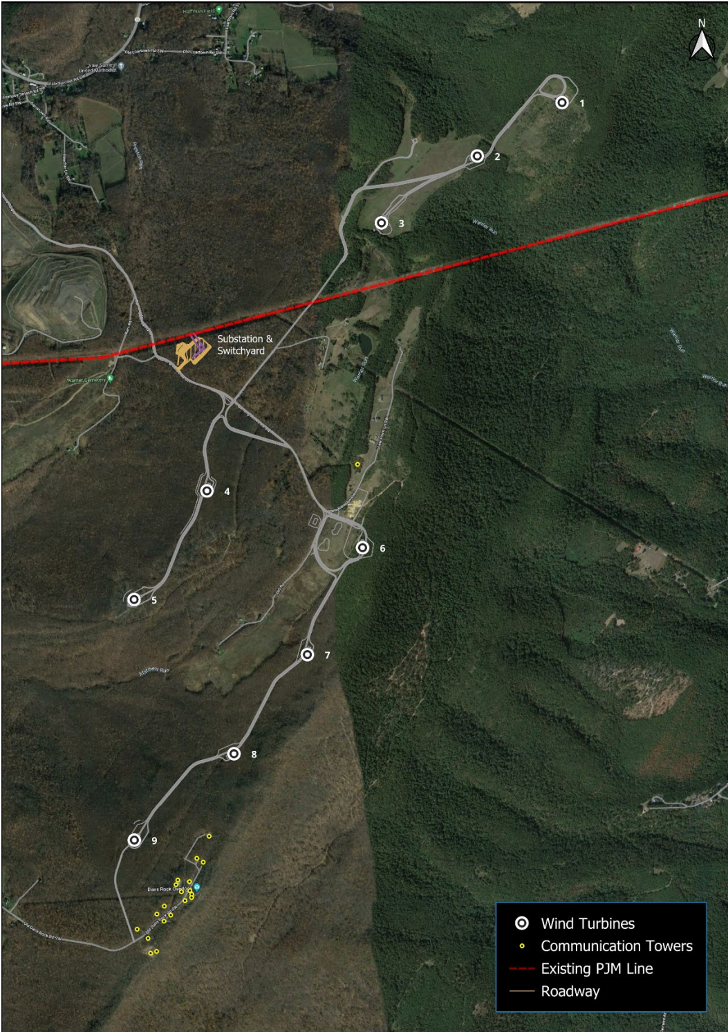
Figure 32. Substation location adjacent to the existing 138 KV transmission line
